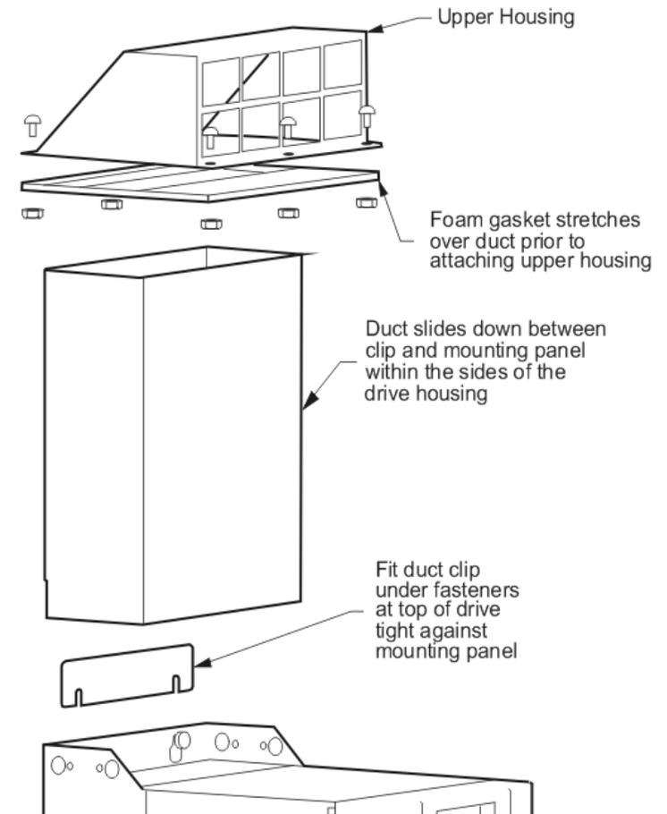
**Figure 3- 3 Frames 4 & 5 External Vent Kit**
