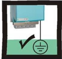
The unit must be **permanently earthed** due to the high earth leakage current.
