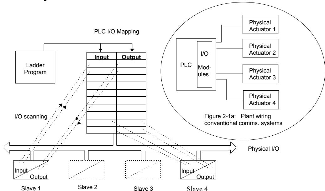
**Figure 2 PROFIBUS compared with conventional comms. systems**
