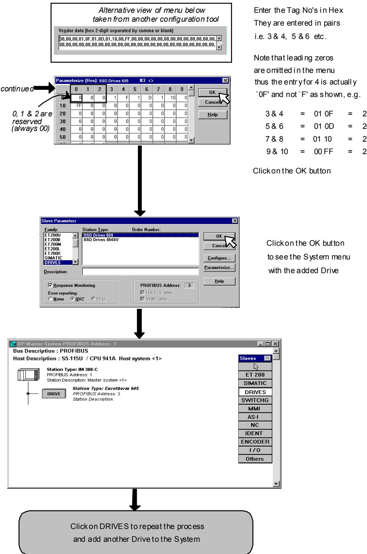
**Figure 9 Typical Configuration Tool Procedure**
