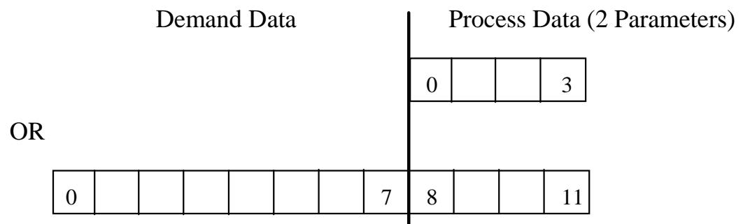
To enable the Demand Data feature, the first byte of Cfg\_Data is set to 0x73 (115 decimal). The number of Inputs and Outputs in the Process Data is defined by setting bytes to either 0x50 (80 decimal) or 0x60 (96 decimal).
