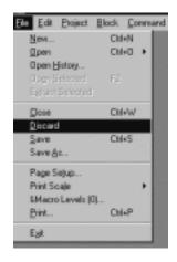
**Discard** allows you to close a configuration without saving. You will lose all of the changes that were made since the configuration was last saved.
