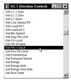
This list shows all the parameters inside the section control block that can be monitored online. To pull up a Monitor list hold the shift key and double click one of the get parameters. The program will then prompt for a name for the Monitor Log file. Click on OK when finished.
