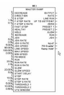
The new *SAM* functions appear on the output side of the blocks, and the connection names have a smaller font, and are followed by an asterisk. They look like regular outputs, but will only function when in a *SAM* mode. An output connection can be tagged to these new outputs and sent out of a macro, for monitoring on the outside of a macro.
