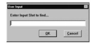
The **Find Input** command will find an Input Slot in the open configuration. Enter the desired slot number and the page with the slot number will appear.
