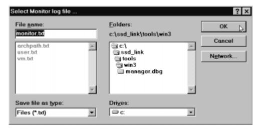
Any information displayed in the Monitor List will be stored in the log file. The Monitor List is the only window where the parameters are updated real time. The number of parameters monitored should be limited to 10-15 total but are not limited to a single address. The Monitor List now has the capability to be saved. To save the Monitor List, make sure it is the active window, by clicking on the title bar.
